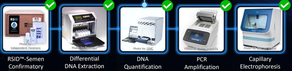
▲ **Figure 9.** Downstream semen confirmatory and STR DNA workflow of the laboratory.
